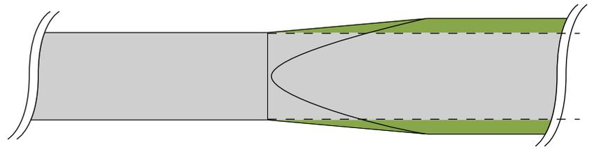
This adaptor has been optimized for increased machining stability with an elliptical shape and a thicker base at the back end.
