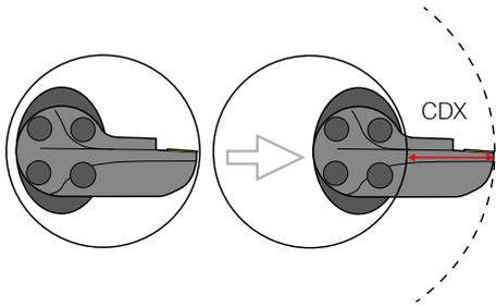
The elliptical shape of the adaptors is optimized for reaching the seat pocket feature. The optimized cutting heads gives you the capacity to reach maximum cutting depth (CDX).
